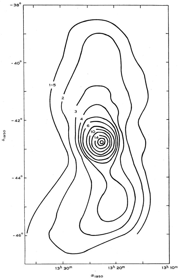
Fig. 1.—Centaurus A at 85.5 Mc/s; aerial beamwidth 50 min of arc. Contour interval, 3000 °K. This chart is similar to one published by Sheridan (1958), but differs in minor details. It is based on Sheridan's observations but includes quantitative beam-asymmetry corrections.
