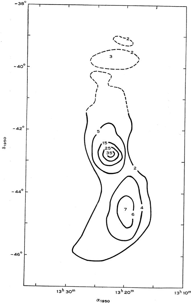
Fig. 2.—Centaurus A at 1400 Mc/s; aerial beamwidth 36 min of arc. Contours are marked in degrees of aerial temperature. These are preliminary observations made by D. S. Heeschen with the 85-ft radio telescope at the National Radio Astronomy Observatory (Green Bank, West Virginia), and they are reproduced here with his permission.
