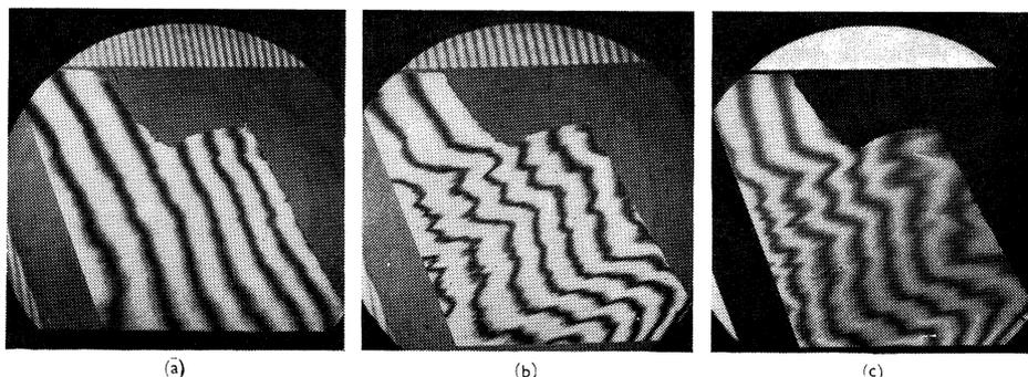
Fig. 3.—Optical quality of one of the calcite crystals with plane parallel faces. (a) Interference fringes, ordinary ray. (b) Interference fringes, extraordinary ray. (c) Birefringent fringes (see text).
