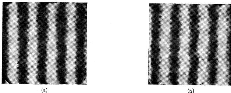
Fig. 5.—Birefringent fringes (double transmission) of each of the two thickest (46 mm) calcite components. A thin supplementary quartz wedge provides several fringes across the surface. The right-hand component is the worst in the whole filter.
