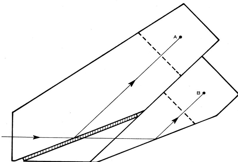
Fig. 6.—Polarizing beam-splitter. A plate of calcite (hatched), with its optic axis perpendicular to the plane of the diagram, is sandwiched between glass prisms, the extraordinary ray being reflected and the ordinary ray transmitted. Faces at 45° reflect the two rays upwards (perpendicular to the plane of the diagram) at *A* and *B*, the dimensions being such that the two images are in focus simultaneously on a plane parallel to that of the diagram.
