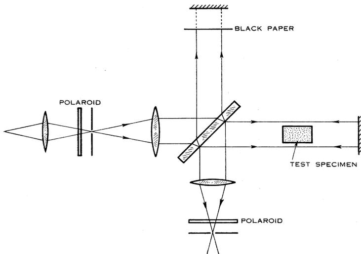
Fig. 4.—Twyman interferometer modified for viewing birefringent fringes. Polarizers are inserted before the entrance pupil and near the eye, with axes at  $45^\circ$  to those of the test specimen. The comparison mirror is covered with black paper.
