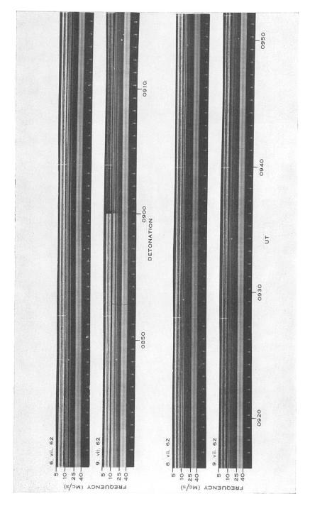
of reception of low frequency signals at the time of detonation on July 9 is clearly seen and the slow recovery of propagation conditions Reception conditions on July 9 compared with those existing on July 6 (the receiver gain was higher on July 9). The abrupt termination can be followed by comparison with the July 6 record.
