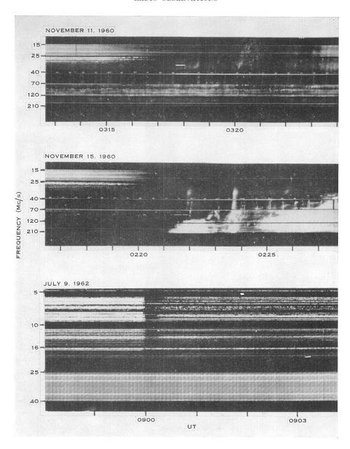
Fade-outs produced by solar flares (top and centre) and the nuclear explosion (bottom). Solar radio emission following the fade-out can be seen in the solar records. The horizontal lines in the 25–40 Mc/s range of the July 9 record are caused by interference from local T.V. transmissions not affected by the ionosphere. (A higher gain setting was used on this range.)
