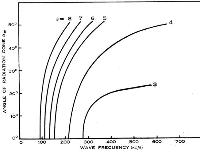
Fig. 7.—Variation of the angular radius  $\alpha_m$  of the emission cones with frequency for a 110 keV electron travelling down the  $60^\circ$  field line.
