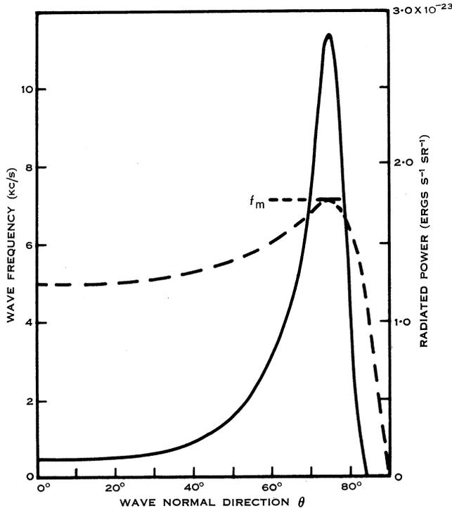
Fig. 1.—Variation of backward Doppler frequency with wave normal direction  $\theta$  (dashed curve) and radiated power with  $\theta$  (solid curve). Electron energy 110 keV; field line latitude  $60^\circ$ ; emission latitude  $30^\circ$ ; scale frequency 500 kc/s.
