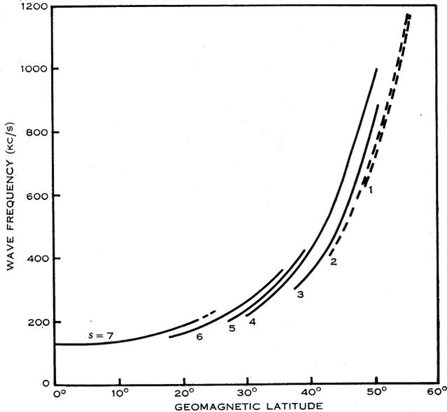
Fig. 6.—Variation of wave frequency with geomagnetic latitude produced by electron bunch travelling along the 60° field line. Solid curves, electron energy 110 keV; dashed curves, electron energy 250 keV.
