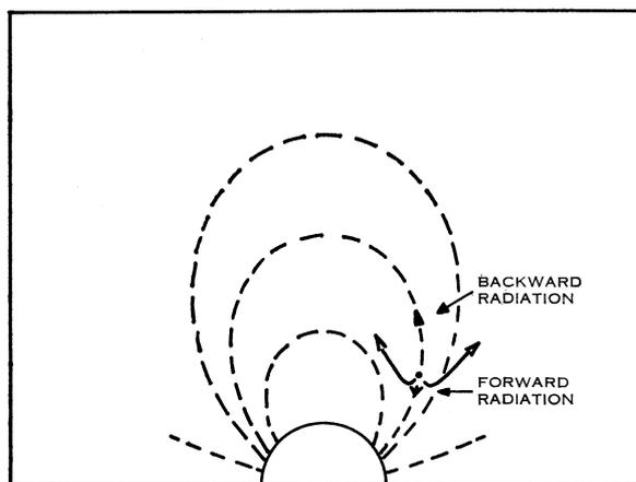
Fig. 8.—Ray paths of the backward and forward radiation.
