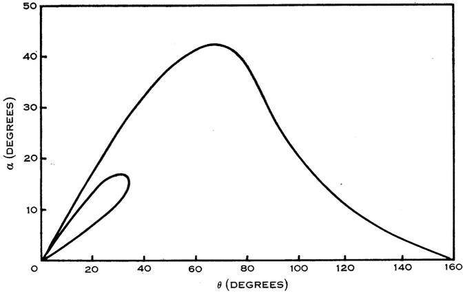
Fig. 4.—Relation between initial direction of wave normal  $\theta$  and final direction  $\alpha$  after refraction by the local plasma. Parameters as in Figure 2.
