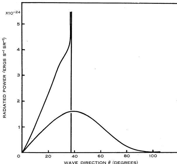
Fig. 3.—Variation of radiated power with  $\theta$  for forward radiation. Parameters as in Figure 2.
