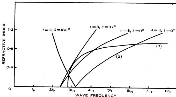
Fig. 2.—Graphical solution of the Doppler equation (2) and the refractive index equation (3) for forward radiation. ( $\lambda = 40^\circ$ ,  $\beta = 0.6$ ,  $\phi = 29^\circ$ ,  $f_H = 100$  kc/s,  $f_0 = 223$  kc/s.)
