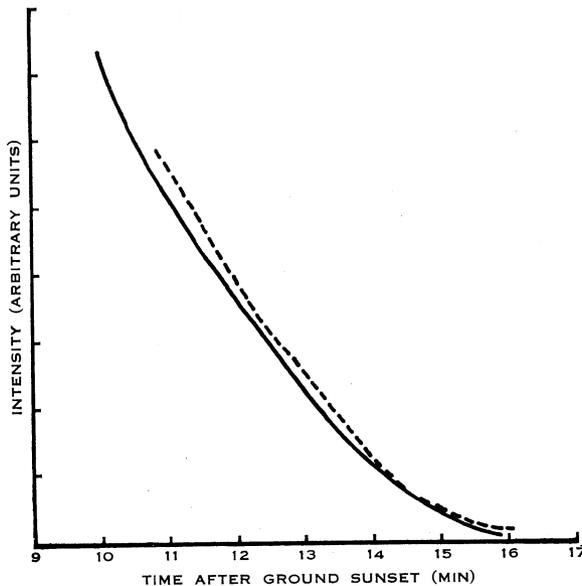
Fig. 4.—Intensity profiles obtained during sunset on May 6, 1964 for the wavelengths  $0.44 \mu$  (---) and  $0.70 \mu$  (—), with the corrections mentioned under Figure 2.
