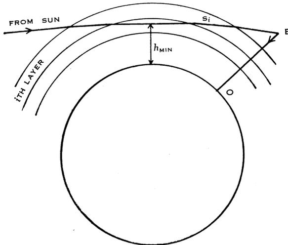
Fig. 1.—A section through the Earth containing the levelled balloon B, vertically above the observer at O (Melbourne, latitude  $38^\circ$  S.), and the path of sunlight traversing a distance  $S_i$  in the  $i$ th layer in the stratosphere.
