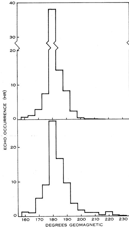
Fig. 4.—Distribution of occurrence of central azimuth values of FAE<sub>d</sub>. U-echoes, upper; P-echoes, lower.
