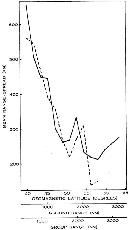
Fig. 8.—Variation of mean range-spread of  $F_{AE_d}$  as a function of geomagnetic latitude, ground range, and group range. P-echoes, solid line; U-echoes, dashed line.
