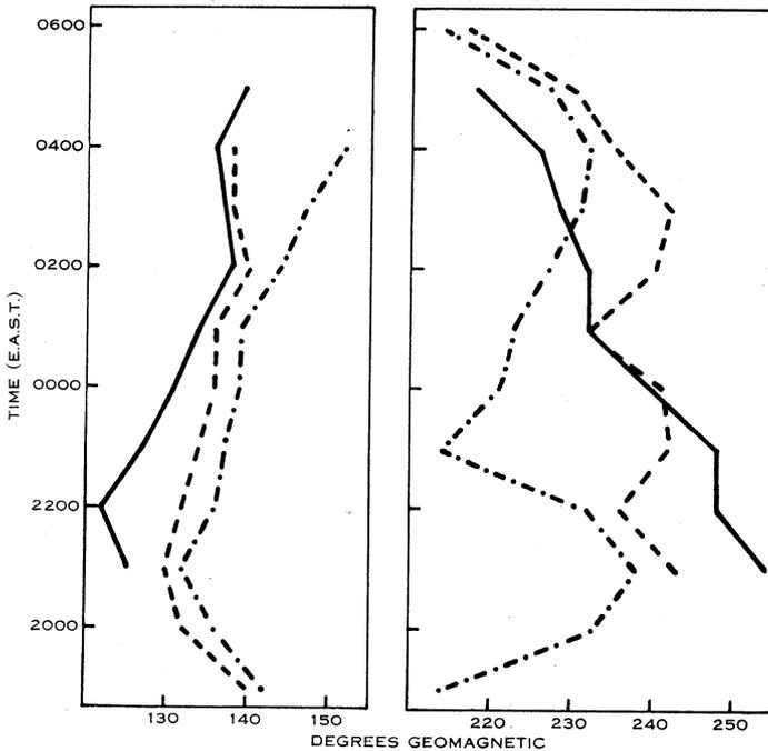
Fig. 5.—Variation of maximum azimuth limits of all  $F A E_d$  with hour of night. Predicted variation, solid line; 5% occurrence level, dashed line; 10% occurrence level, chain line.
