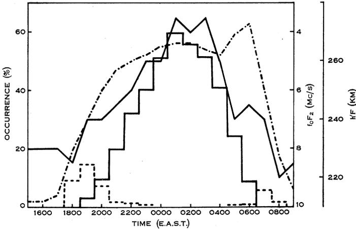
Fig. 2.—Percentage occurrence of FAE as a function of hour of night (histogram).  $\text{FAE}_d$ , solid line;  $\text{FAE}_{1F}$ , dashed line. Also shown is the variation with time of median  $f_0 F_2$  (chain line), plotted inversely, and median  $h'F$  (solid line), both measured at Canberra.
