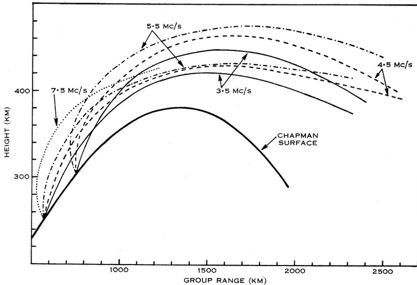
Fig. 9.—Meridian plane sections of various echo surfaces, for a parabolic layer of semi-thickness 100 km, and critical frequencies and base heights as marked. The no-refraction (Chapman) surface is included for comparison. (After Dearden (1962b).)
