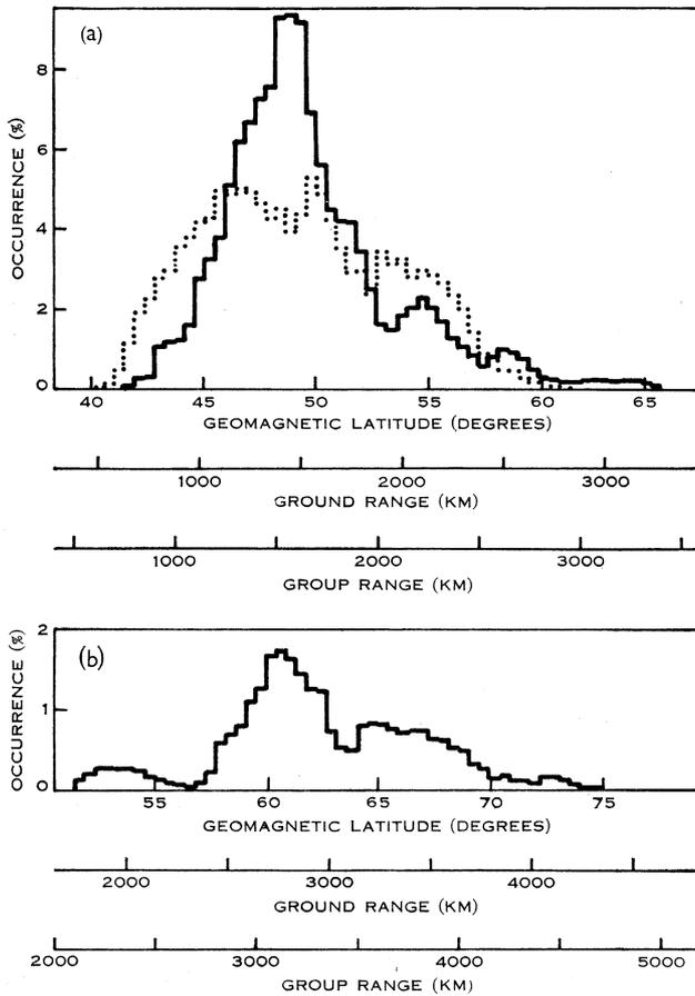
Fig. 1(a).—Percentage occurrence of  $F AE_d$  as a function of geomagnetic latitude, ground range, and group range. P-echoes, solid line; U-echoes, dotted line. An average correction was applied to reduce group range to ground range and latitude.
