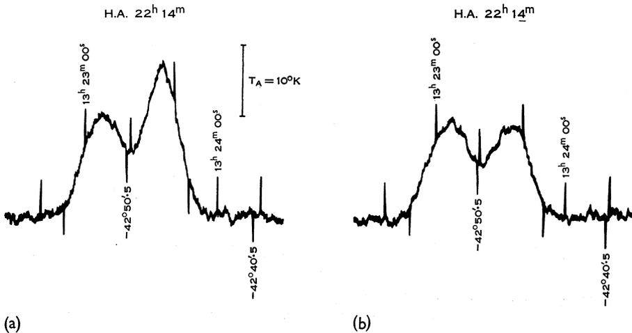
Fig. 2.—Scans through the central double source of Centaurus A from south-west to north-east. (a) Feed horn oriented for maximum signal from the north-east (right-hand) source; position angle of  $E$  vector =  $132^\circ$ . (b) Feed horn oriented for minimum signal from this source; position angle of  $E$  vector =  $42^\circ$ .
