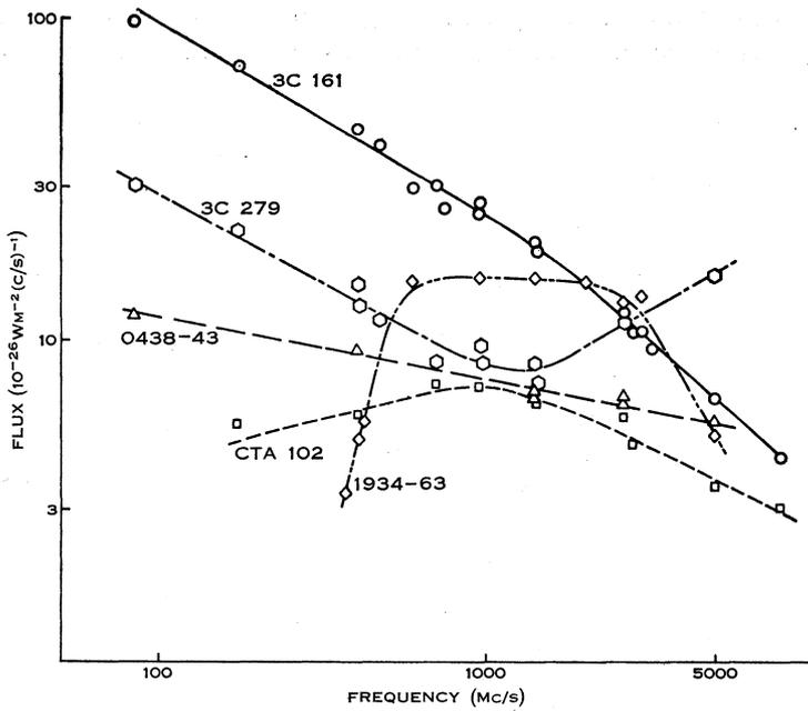
Fig. 1.—Spectra of five radio sources derived from the work of various authors, together with the new 5000-Mc/s observations at Parkes.
