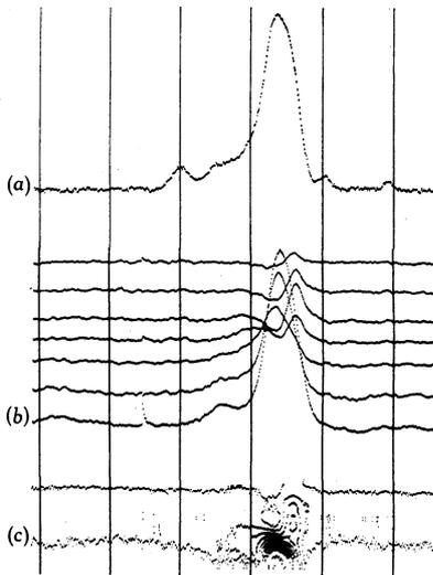
Fig. 1.—A reproduction of one of the Faximile records used in the analysis showing (a) the total power fan beam of the east-west antenna, (b) the seven independent pencil beams of the Cross, and (c) a rough contour map produced in real time. The vertical lines are the 1 min time marks.
