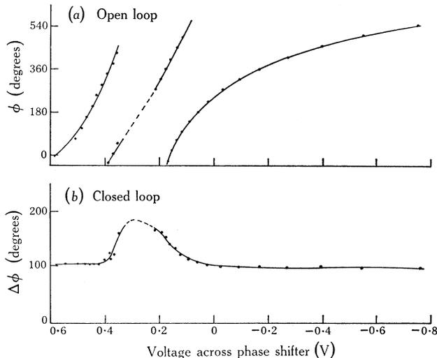
Fig. 3.—Results of the phase-stability test showing (a) the phase error  $\phi$  introduced with change in length of the local oscillator cable and (b) the remaining observed phase change  $\Delta\phi$  after correction by the servo system. The dashed parts of the curves are interpolated values from other similar observations. The zero points of the  $\phi$  and  $\Delta\phi$  scales are arbitrary.
