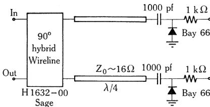
Fig. 2.—Details of the electrical phase shifter used in the phase-stabilizing system shown schematically in Figure 1(b).
