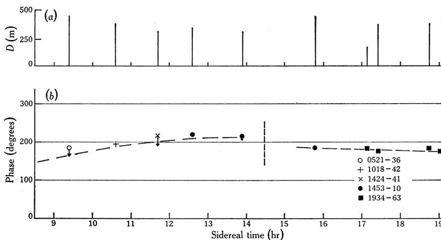
Fig. 4.—Example of a series of phase calibrations showing (a) the track distance  $D$  between the two antennas at which the observations of the indicated calibrating sources have been made and (b) the observed on-line computed phases. The arrows in (b) show subsequent corrections applied to certain measurements, as described in the text, while the dashed vertical line indicates the time of readjustment of the receiving system.
