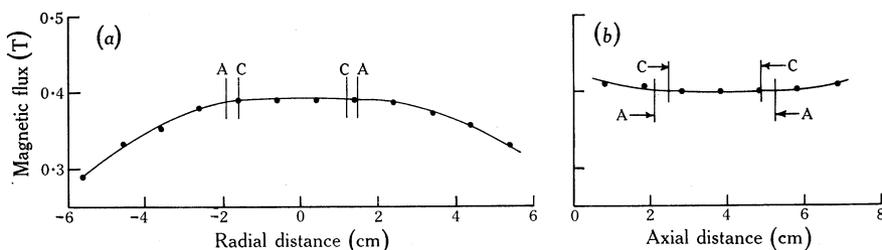
Fig. 2.—Scans of the magnetic field across the gap (a) radially at the mid-pole position and (b) axially along the central axis. The indicated positions of the anode A and cathode C show the interelectrode working volume.
