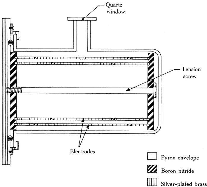
Fig. 1.—Schematic diagram of the ionization chamber.
