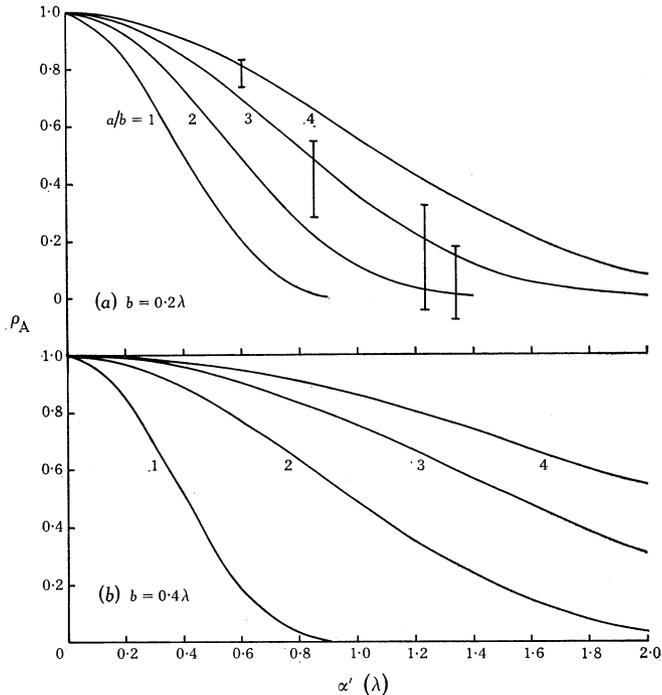
Fig. 1.—Experimental and theoretical plots of the autocorrelation  $\rho_A$  for backscattering from Gaussian irregularities, shown as functions of the receiver separation  $\alpha'$ , the indicated axial ratios  $a/b$ , and the vertical scales (a)  $0.2\lambda$  and (b)  $0.4\lambda$ . The vertical bars in (a) indicate the range of observed values at given receiver separations.
