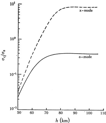
Fig. 2.—Variation with altitude  $h$  of both the ordinary and extraordinary mode scattering cross sections  $\sigma_c$  at 2.4 MHz relative to the cross sections  $\sigma_0$  in the high frequency limit.
