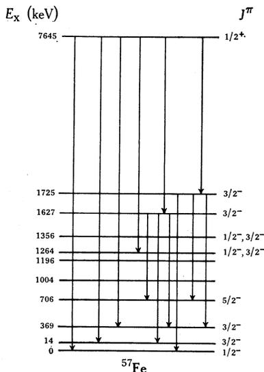
**Fig. 1.** Partial decay scheme of  $^{57}\text{Fe}$  following thermal neutron capture in  $^{56}\text{Fe}$ . Only secondary  $\gamma$ -rays from the 1627 and 1725 keV levels are shown.
