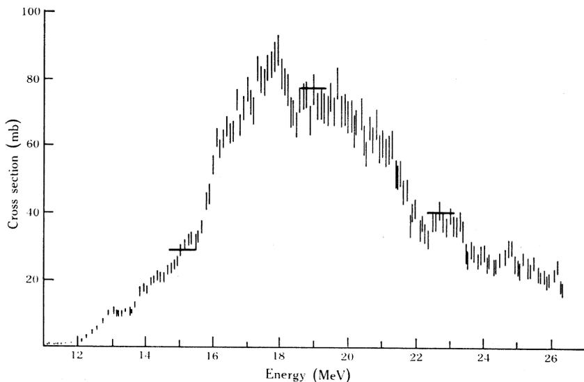
Fig. 1. Photoneutron cross section for natural chromium. The bold horizontal bars represent the analysis bin widths used.
