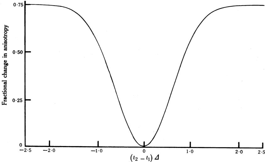
Fig. 3. Calculated dependence of the fractional change in  $\gamma$ -ray radiation anisotropy after a triple-pulse ( $90^\circ$ ,  $180^\circ$ ,  $90^\circ$ ) sequence upon  $(t_2 - t_1)\Delta$ . This is the theoretical spin-echo nuclear orientation lineshape.
