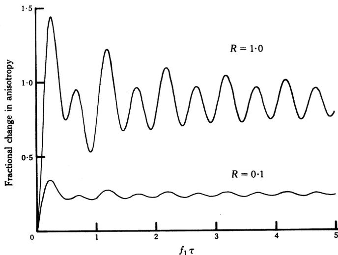
Fig. 1. Theoretical dependence of the signal on  $f_1 \tau$  (where  $f_1 = \omega_1/2\pi$ ) for an inhomogeneously broadened line. The ordinate is the fractional change in anisotropy of the  $\gamma$ -ray radiation. The two curves are for the indicated values of  $R = \omega_1/\Delta$ .
