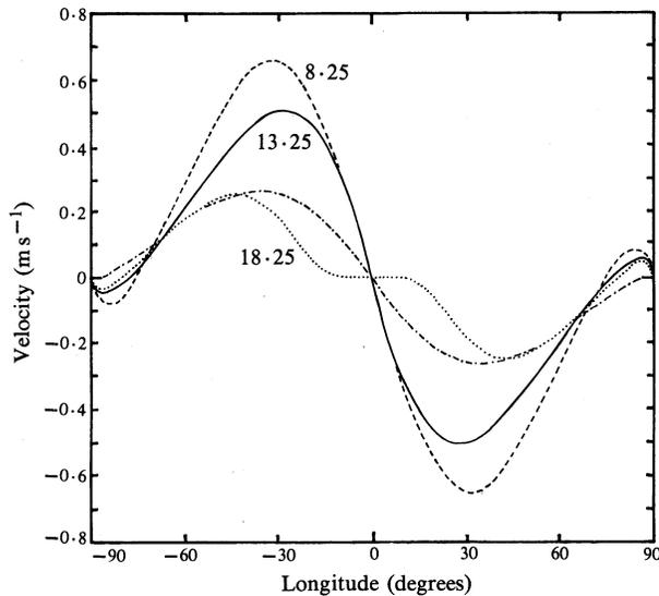
**Fig. 1.** Global velocity modulation caused by the passage across the solar disc of a plage of area 1224 millionths of a hemisphere and a spot area of 122 millionths (dot-dash curve). The plage curves are labelled by the separation (in pm) of the two windows.
