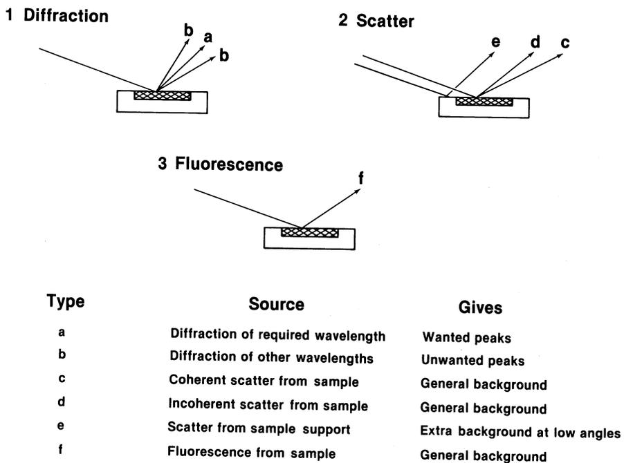
Fig. 1. Composition of a diffraction pattern.
