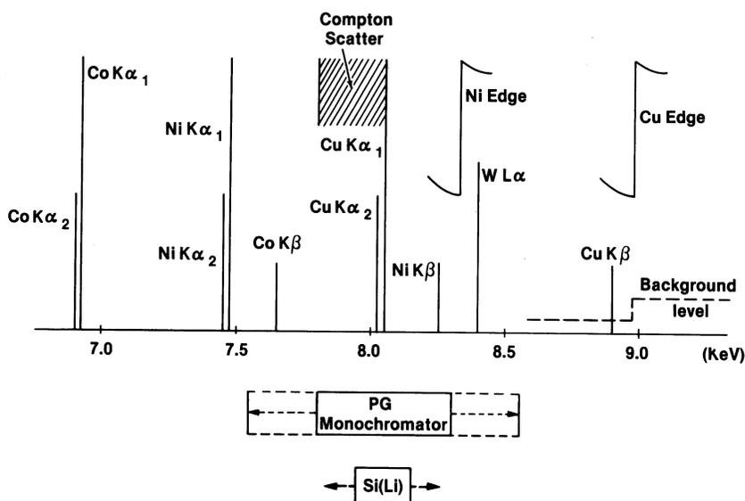
Fig. 2. Bandpass range of a graphite monochromator and a Si(Li) detector.
