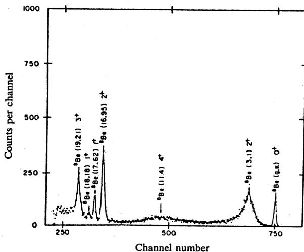
Fig. 3. A deuteron spectrum from  ${}^9\text{Be}(p, d){}^8\text{Be}$  with  $E_p = 33.6$  MeV and  $\theta_{\text{lab}} = 60^\circ$  (from Kull 1967).
