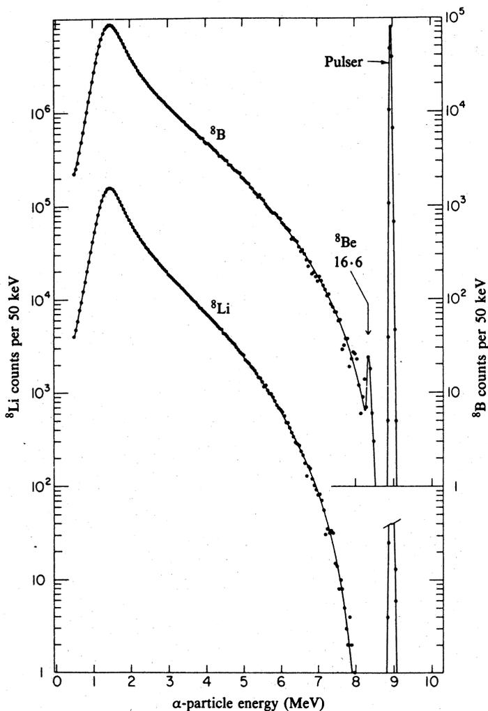
Fig. 8. The  $\alpha$ -spectra from  ${}^8\text{Li}(\beta^-){}^8\text{Be}(\alpha){}^4\text{He}$  and  ${}^8\text{B}(\beta^+){}^8\text{Be}(\alpha){}^4\text{He}$  measured by Wilkinson and Alburger (1971). The solid curves are drawn to guide the eye. [From Warburton (1986).]
