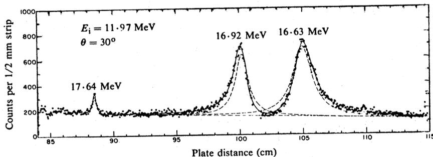
Fig. 6. An  $\alpha$ -spectrum from  $^{10}\text{B}(d, \alpha)^8\text{Be}$  (from Browne *et al.* 1966). The solid curve is a two-level fit to the experimental points (see Section 3). The dashed curves show the shape and position that would have been observed for each level in isolation.
