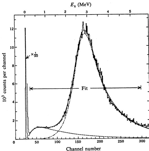
Fig. 7. Calculated (solid curve) and measured (histogram) spectra of deuterons at  $10^\circ$  from  ${}^9\text{Be}(p, d){}^8\text{Be}$  with  $E_p = 39.91$  MeV (from Barker *et al.* 1976). The  $l = 0$  and 2 components of the calculated curve are plotted as dashes and dot-dashes respectively. The  $l = 0$  component is normalised to the ground state main peak.
