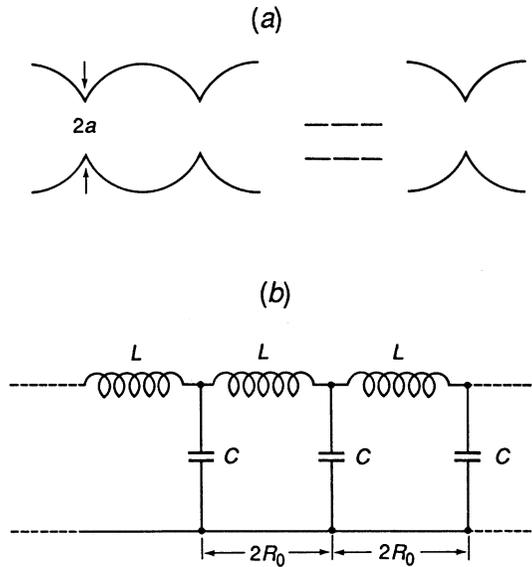
**Fig. 1.** Linear array of identical spheres, each of radius  $R_0$ , and with interparticle contact radius  $a$ . (b) Equivalent electrical transmission line.
