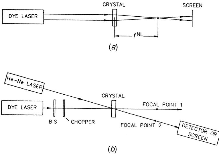
**Fig. 1.** Experimental set-up for the measurement (a) of focal length and (b) of the response time, where BS is a beam splitter.
