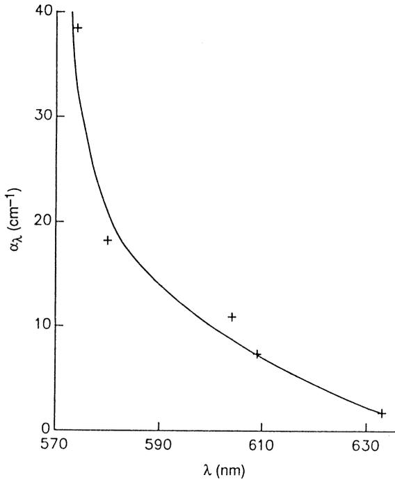
**Fig. 3.** Relationship between the measured absorption coefficient  $\alpha_\lambda$  and the operating wavelength  $\lambda$ .
