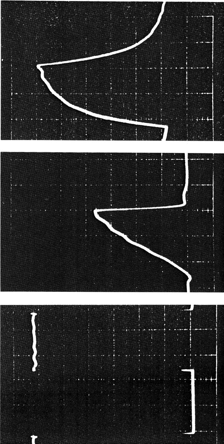
**Fig. 5.** The input dye laser pulses (a) and the traversing probe He-Ne laser pulses: (b)  $I = 60$  mW and (c) 20 mW. The units on the abscissa are 50 ms/div.
