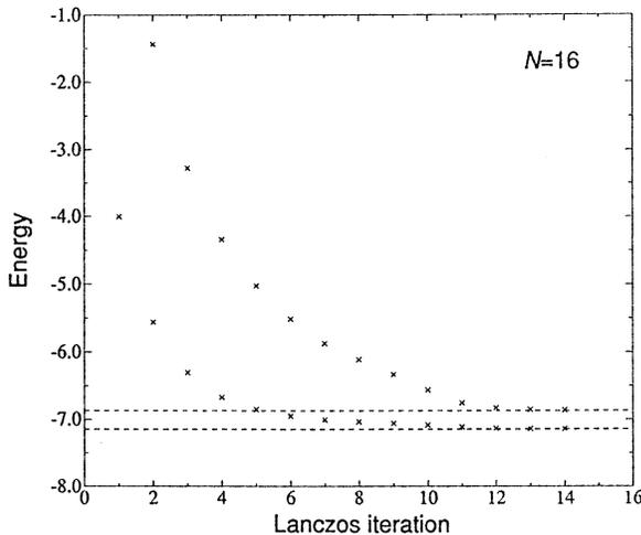
**Fig. 1.** Convergence of the ground and first excited states for  $N = 16$  with the Néel state as the trial state. The exact values of the ground and first excited states are shown as dashed lines. Hamiltonian moments were computed numerically.
