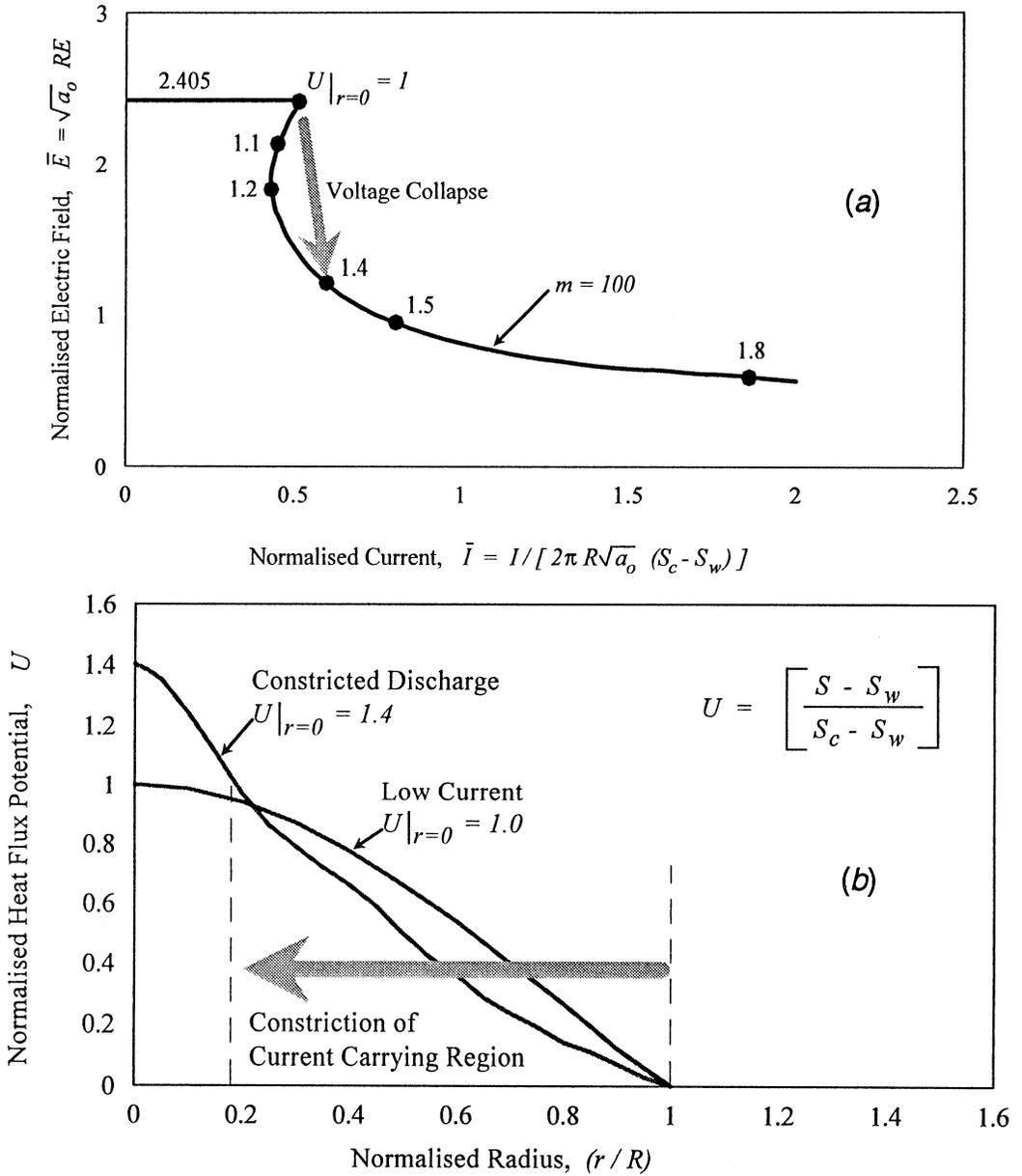
Fig. 5. Voltage collapse and constriction of a cylindrical arc discharge.
