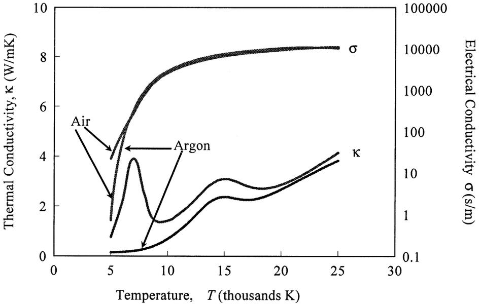
Fig. 3. Variation of electrical and thermal conductivities of plasmas with temperature.
