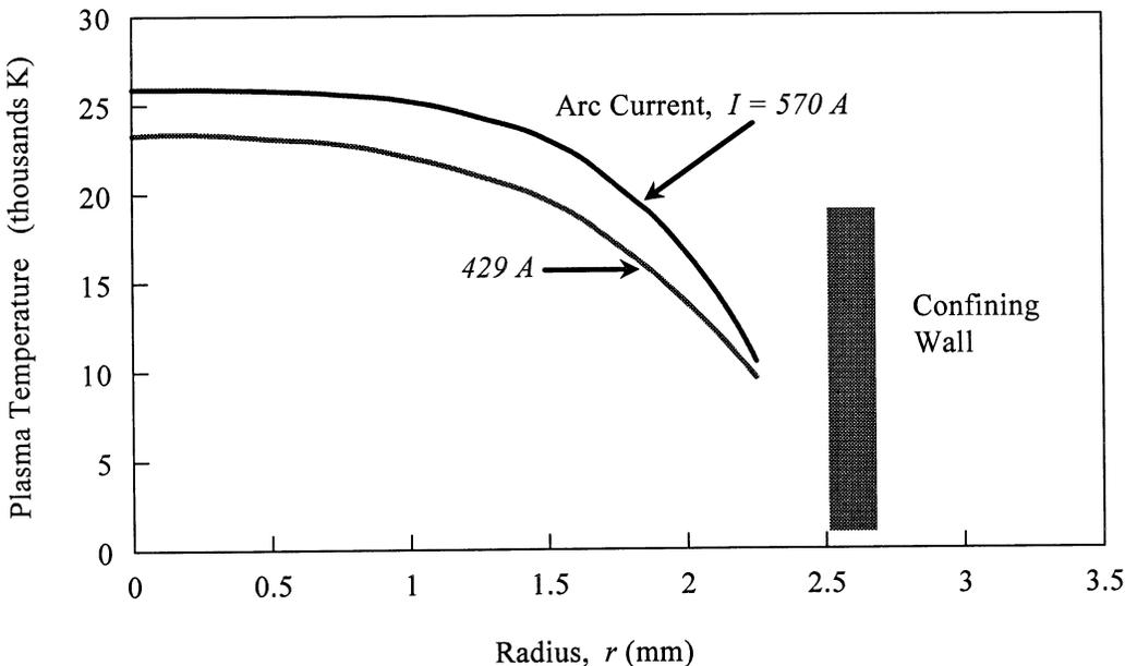
Fig. 6. Temperature profiles of wall-stabilised nitrogen arcs.
