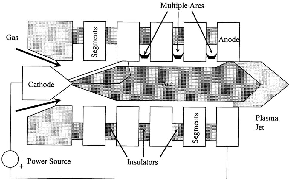
Fig. 13. Torch with segmented/cascade nozzle for fixed-length arc operation.
