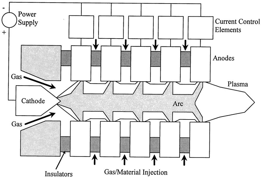
Fig. 14. Electronic plasma torch with multiple anodes for power control.
