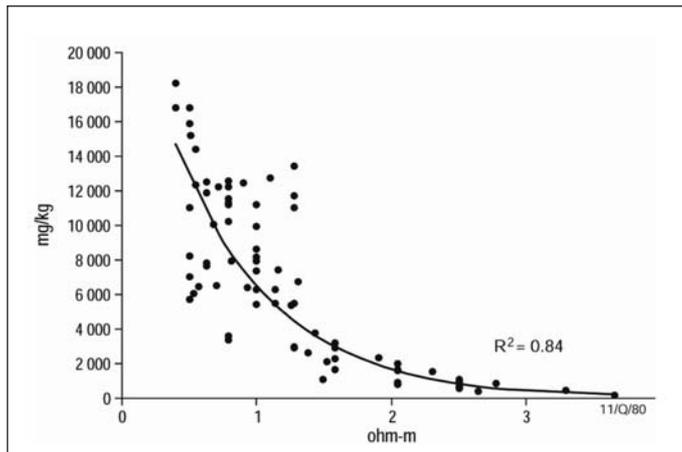
Fig. 5. Scatter plot of NanoTEM® resistivity (ohm-m; the inverse of conductivity) and concentration of soluble chloride (mg/kg) as measured in boreholes along the NanoTEM® traverses. The R-squared value of 0.84 indicates that the relationship between the quantity of soluble chloride present in the soil and the electrical conductivity is very strong. (An R-squared value of 0.84 implies that variations in the soluble chloride concentration explain 84% of the variation in the NanoTEM® response).
