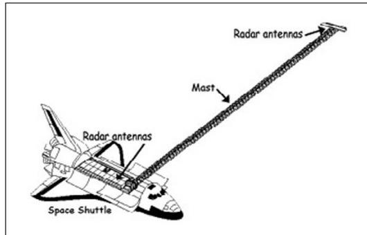
Fig. 1. The SRTM dual radar antenna setup on the Shuttle spacecraft.
