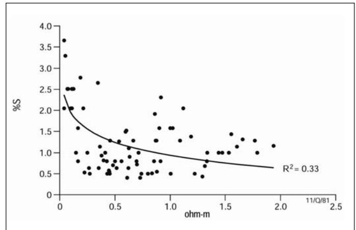
Fig. 6. Scatter plot of NanoTEM® resistivity and potential acidity (the percentage of sulfide present in the soil). The resulting R-squared value of around 0.33 irrespective of the trend/regression type applied suggests there is little, if any, relationship between the electrical conductivity and sulfide content in the Pimpama study area.
