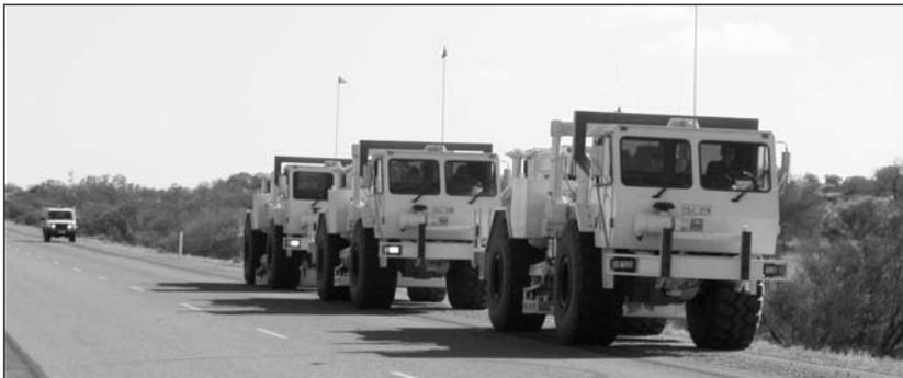
Fig. 2. The source Vibroseis trucks operating on the Woomera to Roxby Downs road.
