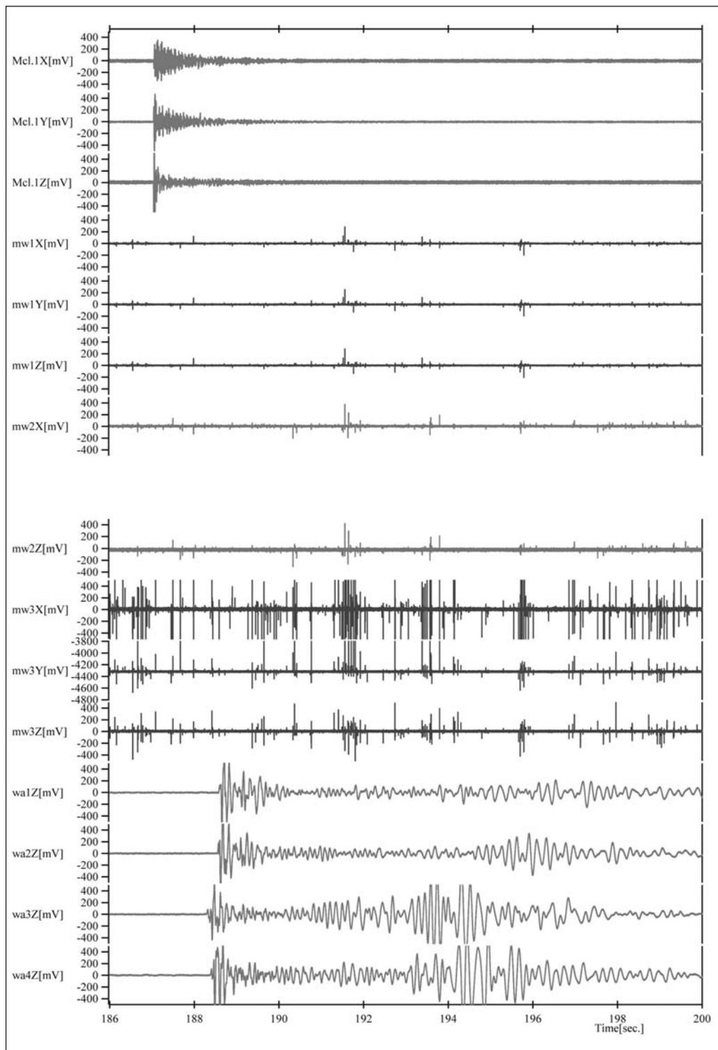
Fig. 5. Seismograms of seismic event originating from close to Habanero-1.
