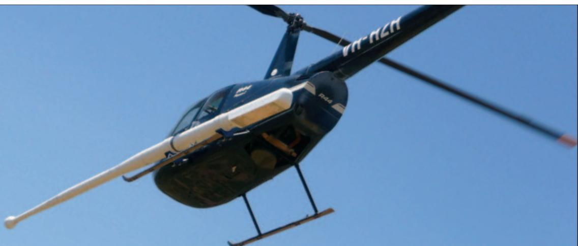
World first piston engine helicopter stinger installation for low cost, high quality airborne radiometric and magnetic data collection
