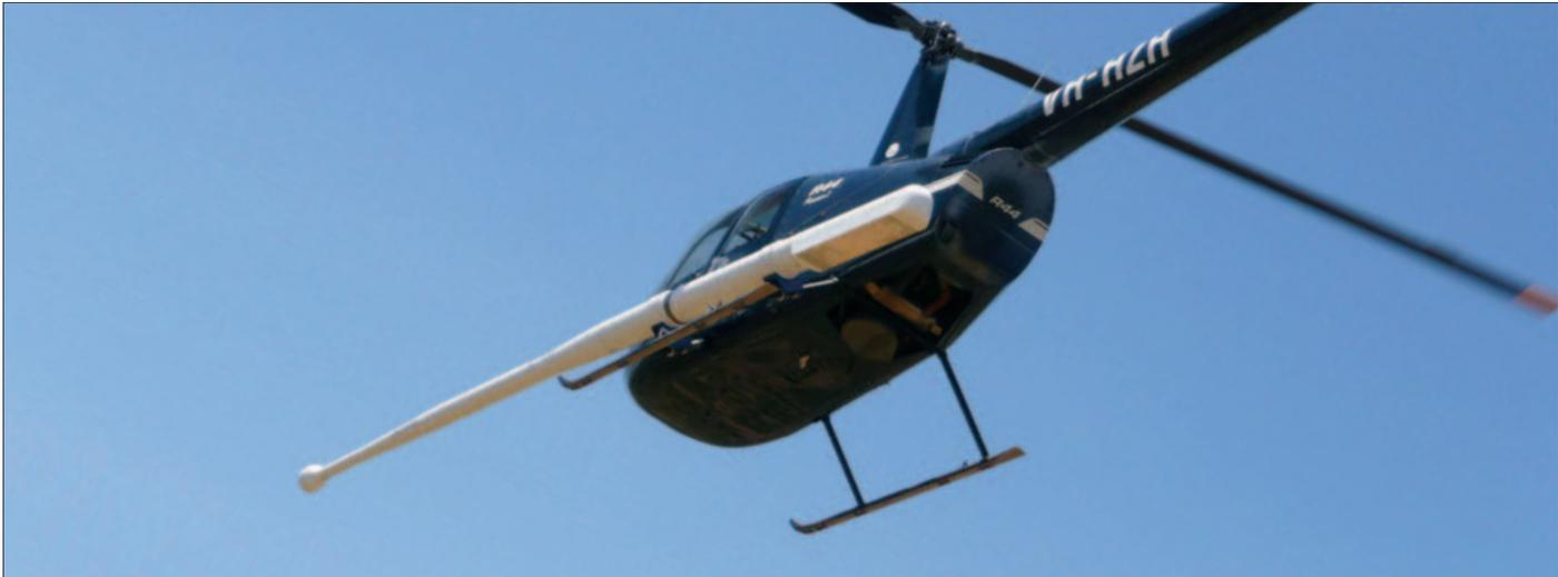
World first piston engine helicopter stinger installation for low cost, high quality airborne radiometric and magnetic data collection
