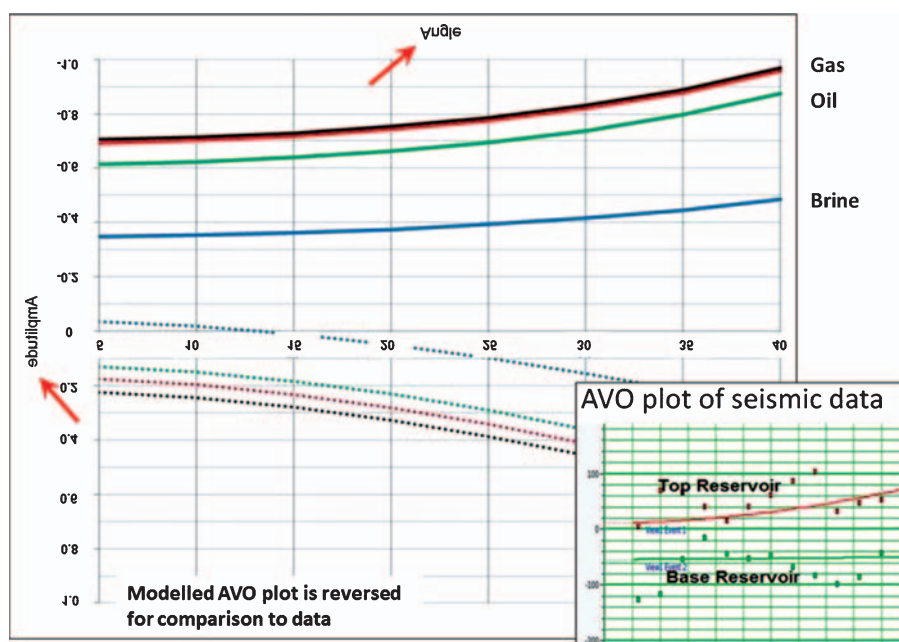
Fig. 3. Example of AVO modelling results presented by an Australian operator. For comparison the display of modelled results has been inverted to account for the negative polarity convention of the seismic data (lower right). Inverting the graphical display to match the measured seismic response results in unreadable text (arrows).
