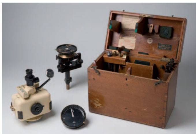
Fig. 1. Watts variometer no. 15887, dating 1935. Implementation: Used on AGGSNA survey of Tennant Creek (1935) and later on Cocos Island (1946) and Macquarie Island (1950–52). Image: National Museum of Australia, 2007.
