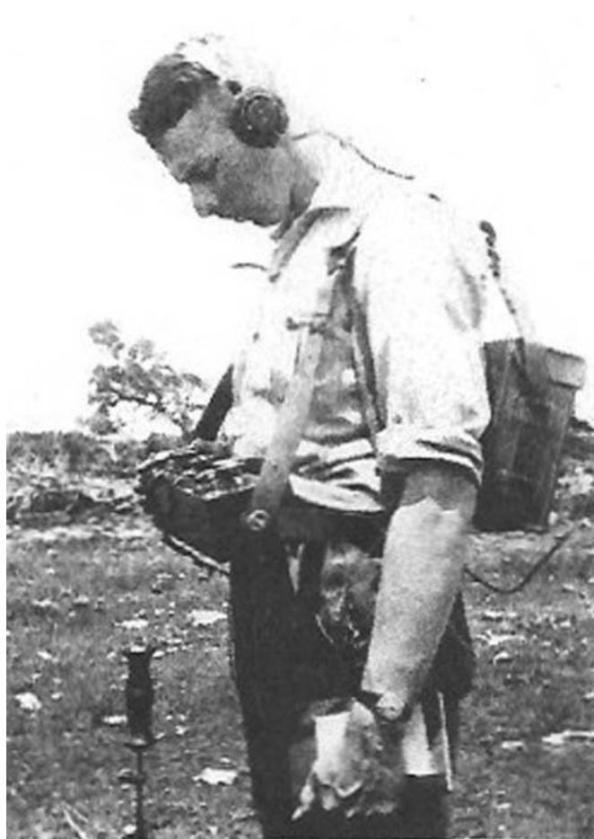
Figure 2. A photo of the ratiometer in use with headphones and an amplifier on the operator's back (from Broughton Edge and Laby, 1931, Fig. 33).
