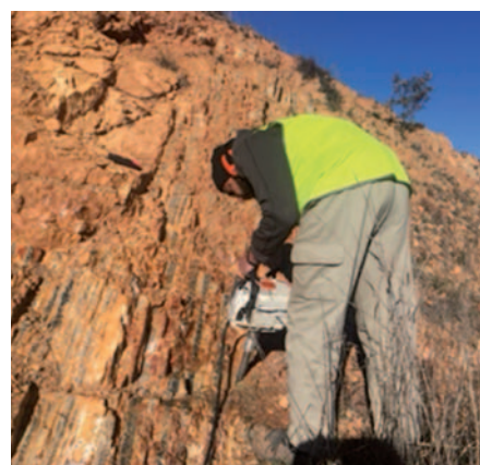
Figure 3. PhD student Umer Habib coring siltstone in the Rockley Volcanics.
