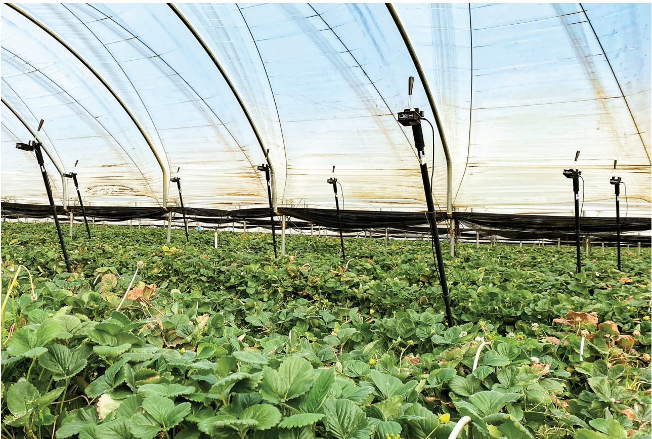
Figure 3: Raspberry Pi-based video capture units placed over strawberry vegetation (locations indicative only).
