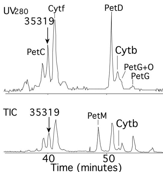
**Figure 1.** LCMS+ of spinach cytochrome *b<sub>6</sub>f* subunits. A reverse-phase separation is eluted directly to an electrospray-ionization mass spectrometer with a split line allowing simultaneous collection of fractions. Cytochrome *b* elutes with low efficiency just before singly oxidized PetG.
