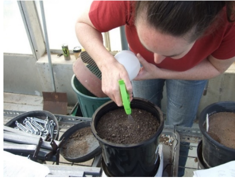
Figure S6. Photograph showing spray application of the polymer formulation on to pots in the glasshouse. Credit: Dr Michael Braunack (CSIRO Agriculture and Food).
