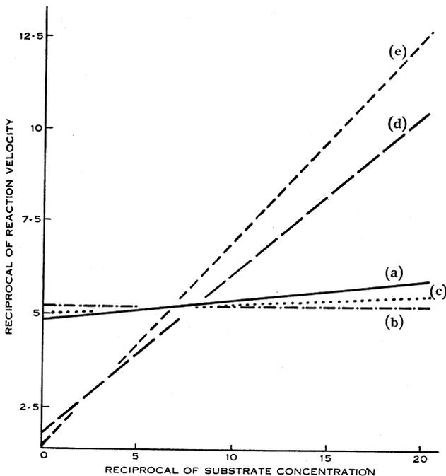
Fig. 9.—Effect of higher concentrations of glycerol on the hydrolysis of *p*-nitrophenyl- $\beta$ -glucoside by *S. atra*  $\beta$ -glucosidase. (a) No addition. (b) 1.0M Glycerol. (c) 1.5M Glycerol. (d) 1.75M Glycerol. (e) 2.0M Glycerol. Unit substrate concentration  $2 \times 10^{-3}$ M.
