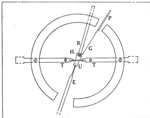
Fig. 1.—The experimental chamber in which single bladders of *Utricularia* sp. were mounted in FPW. The bladder *U* was held by its stem between two Perspex tweezers *T*. A Perspex rod *R* was used to prevent forward movement of the bladder during the insertion of a pressure-measuring capillary or microelectrode *E*. A fine glass probe *G*, attached to a 20-mm strip of piezoelectric material *P*, was positioned near one of the sensitive hairs *H*.
