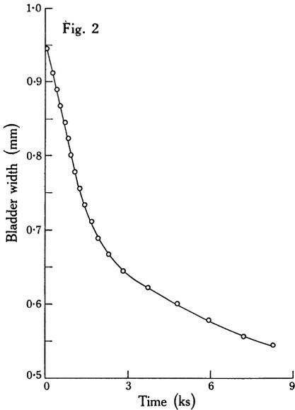
Fig. 2.—Change in width of a bladder as a function of time after firing.
