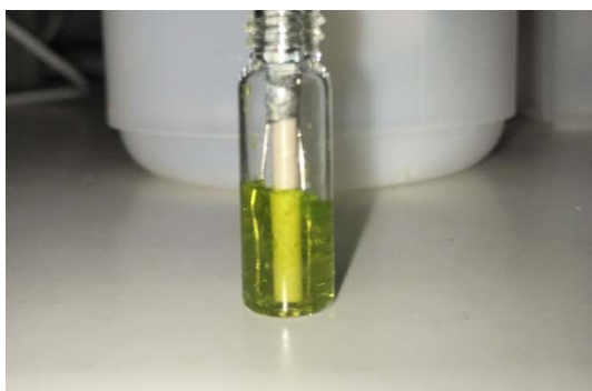
Figure S7. 3-electrode cell used for Diffusion coefficient and Cyclic voltammetry experiments
