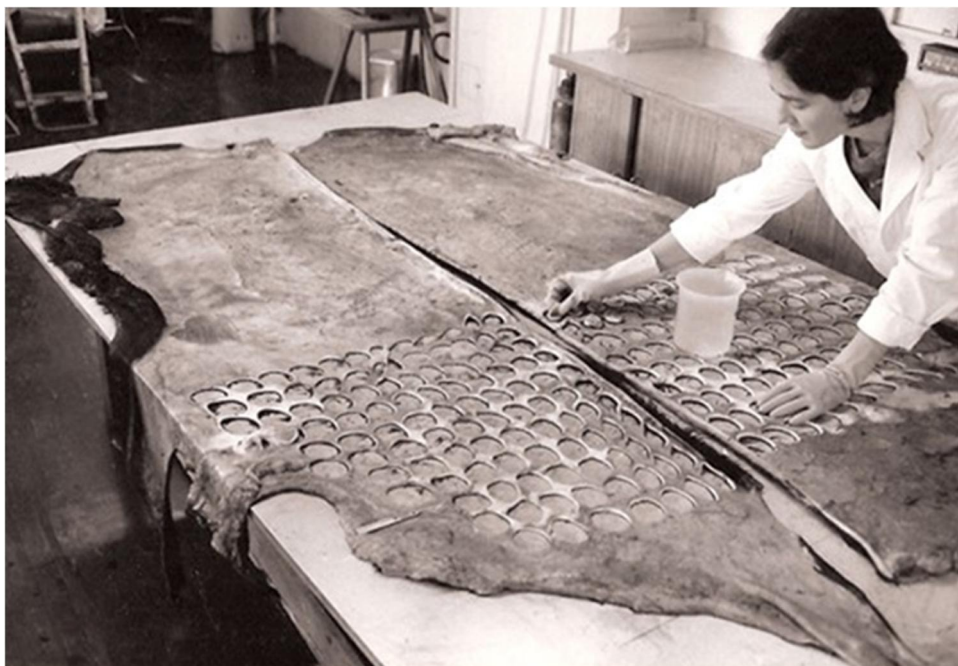
Fig. 7. Catherine Money cutting hide samples for laboratory preservation trials, 1969 [Source: Catherine Money, CSIRO].
