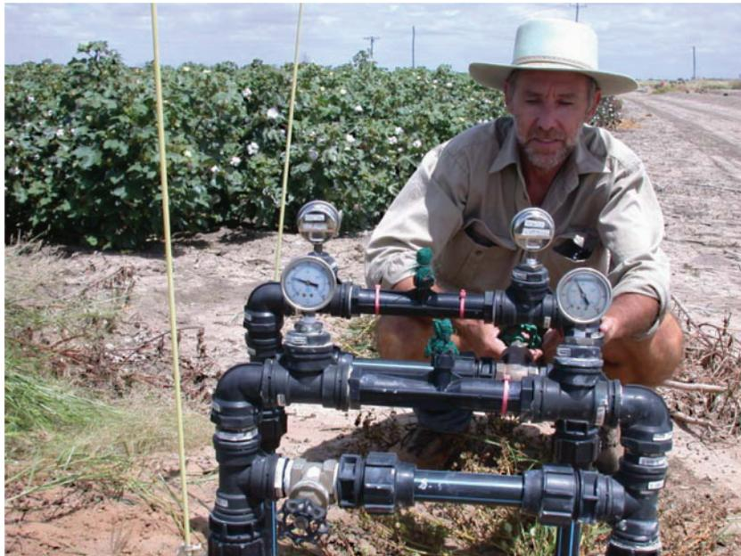
**Fig. 2.** Air-injector (Mazzei Model MI-1583) retro-fitted to existing subsurface drip irrigation system, into individual plot delivery lines before the first lateral take-off point in the irrigation setup.
