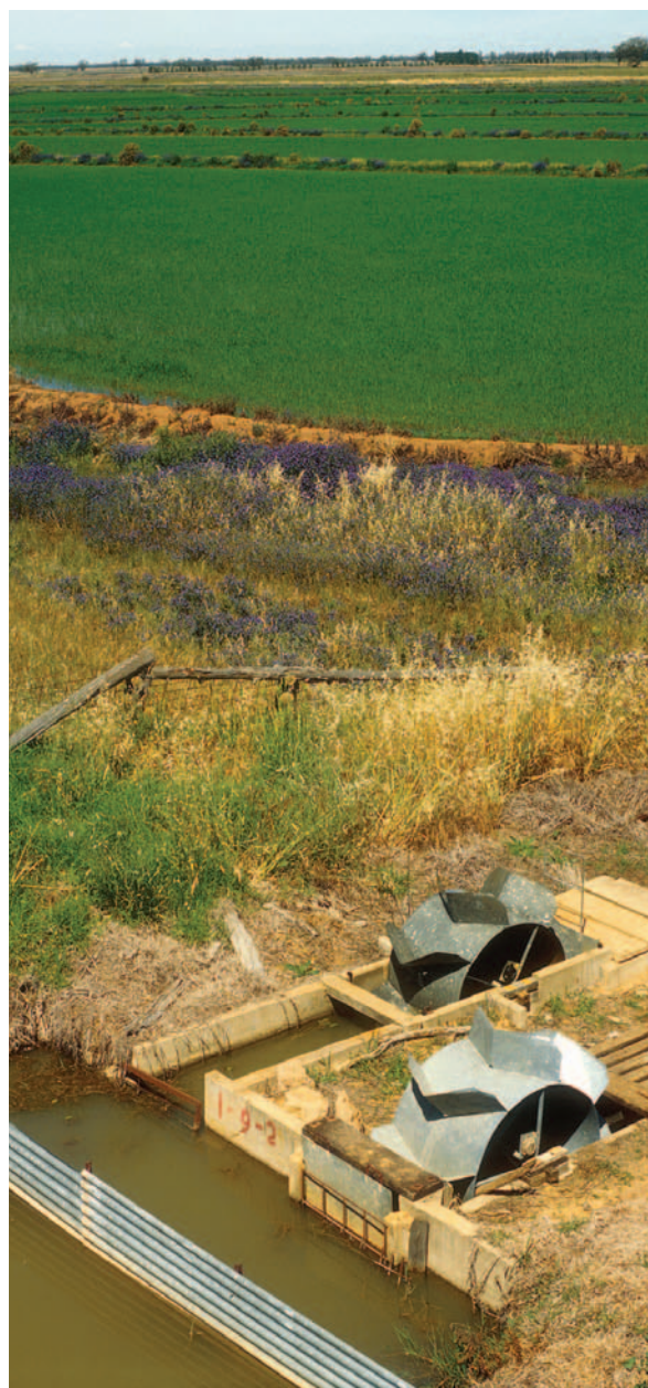
Dethridge wheel measuring irrigation water consumption, Griffith, New South Wales. Photo: Bill van Aken, CSIRO.
