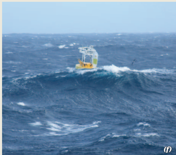
Sampling devices used within the Integrated Marine Observing System. (a) Argo float deployment; (b) autonomous underwater vehicle; (c) acoustic receiver mooring; (d) ocean glider; (e) polynya ocean monitoring; (f) Southern Ocean flux station buoy. Photos: (a) Alicia Navidad, CSIRO; (b) Kim Brooks, AIMS; (c) Rob Harcourt, Macquarie University; (d) Daniel Wisdom, AIMS; (e) Steve Rintoul, CSIRO; (f) Eric Schulz, Bureau of Meteorology.
