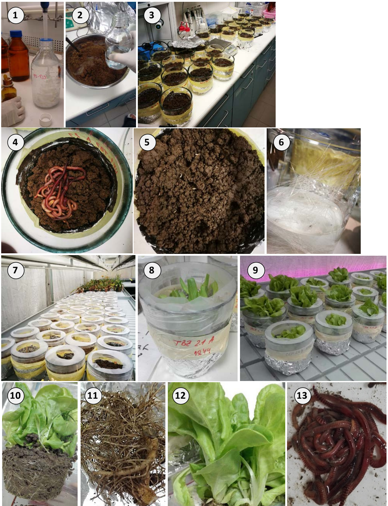
Figure S2: The photos from the experiment. 1) mixing the spiking solutions (CLP-CF); 2) spiking the soil; 3) establishing the microcosms; 4) addition of the earthworms; 5) addition of the lettuce seeds; 6) the SPME fibers cleaned; 7) start in the greenhouse; 8) the detailed view on the microcosm; 9) the microcosms with the grown lettuce; 10)-12) sampling at the time point
