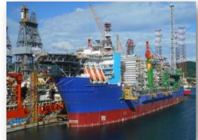
Ichthys Venturer - floating production, storage and offloading facility (FPSO)
