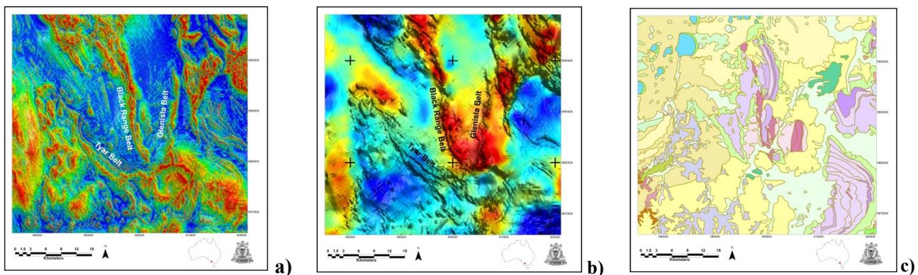
**Figure 1. Images of filtered regional geophysical data and surface geology over the study area. a) Tilt filtered TMI (RTP); b) pseudocolour of 30km high pass filtered Bouguer gravity (red – high; blue - low), overlain on TMI intensity with NE sun-shading; c) 1:250k surface geology showing exposed slivers of Cambrian volcanics (dark pink).**
