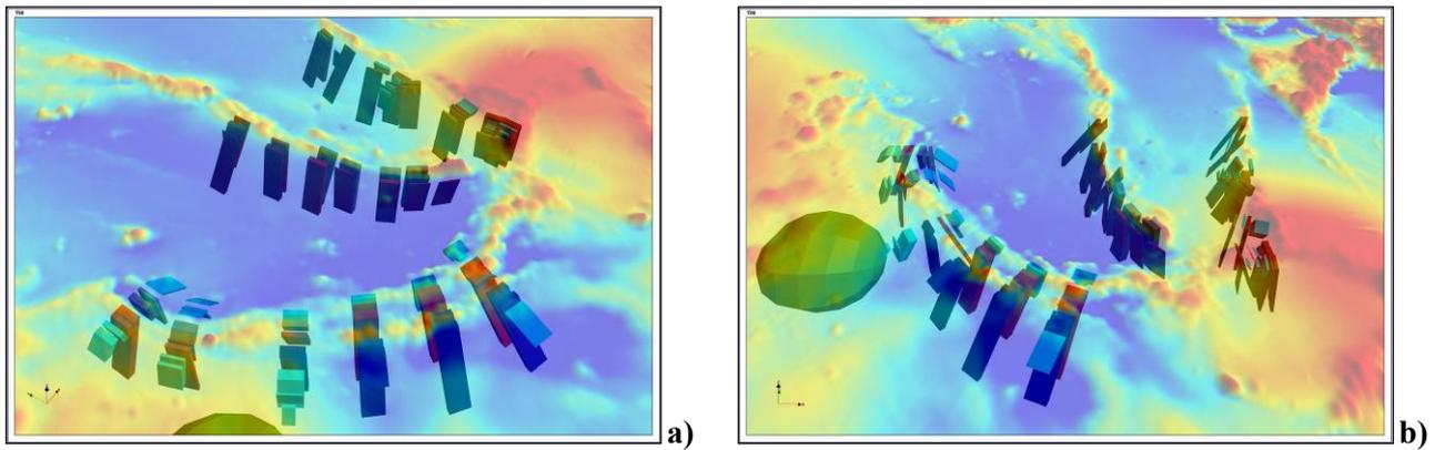
**Figure 3.** 3D perspective views of modelled tabular bodies representing the three segmented Stavely Arc fault slices in the Black Range region, with transparent TMI (RTP) overlay. a) view towards northeast; b) view towards north. Green ellipsoid body to the west represents a buried intrusive – see text.
