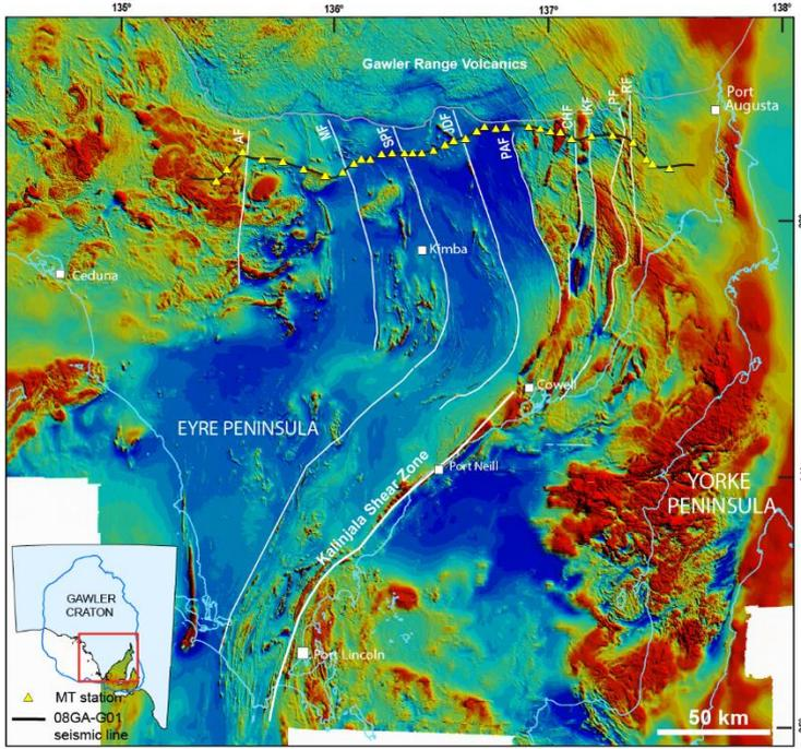
**Figure 1:** TMI image of the southern Gawler Craton, showing the major fault structures. AF=Allalone Fault, MF=Melaleuca Fault, SPF=Shoal Point Fault, JDF=Jungle Dam Fault, PAF=Pickaxe Fault, CHF=Camel Hill Fault, IKF=Iron Knob Fault, PF=Pankalla Fault, RF=Roopena Fault
