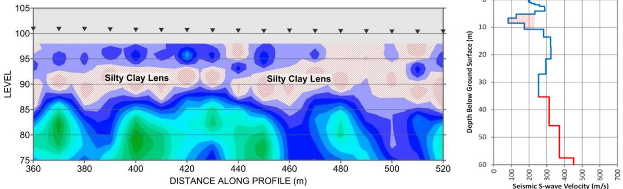
**Figure 5: Sub-section of a generated S-wave velocity section (Figure 4) showing areas of low modelled Vs corresponding to interpreted silty clay lenses. Vs sounding through one of the lenses is shown on the right.**
