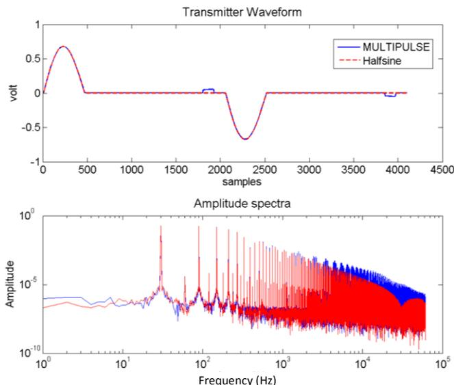
**Figure 1: Current waveform for a halfsine-only pulse (red) and MultiPulse (top panel) and their calculated power spectra (bottom). At low frequencies, the power spectra are the same but at high frequencies (> 2 kHz) the MultiPulse waveform has significantly more power.**
