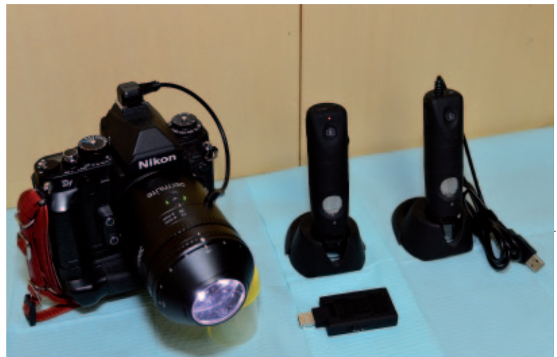
Figure 1. Small hand-held dermoscopes are not adequate for dermoscope-guided surgical procedures. This figure shows the dermoscopes used by us. The left-sided dermoscopy is in the shape of a camera-lens to be mounted on a single-lens reflect camera. This is adequate for assessments and documentations before and after the procedures. The middle (wireless) and right dermoscopes (with wires) are suitable during dermoscope-guided surgical procedures.
