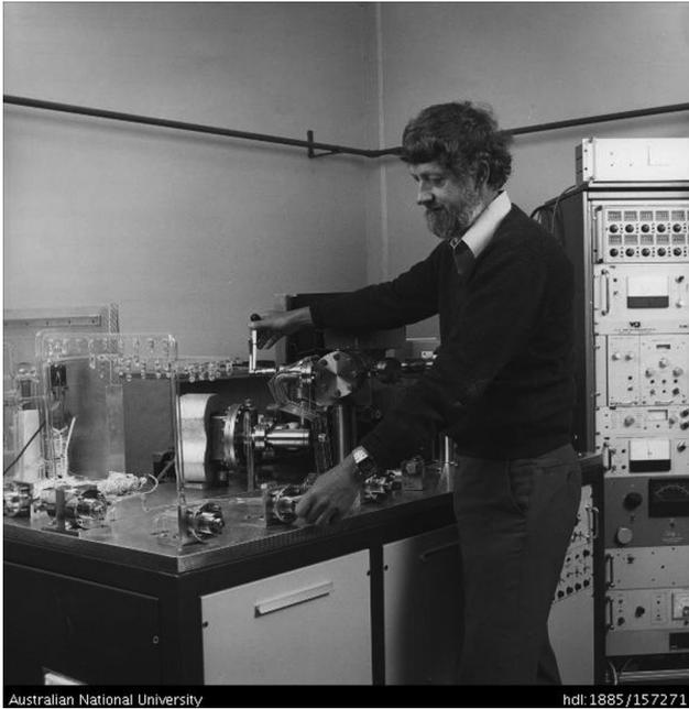
**Fig. 2.** Ian McDougall operating the MS-10 mass spectrometer used for K-Ar dating analyses (circa 1980) (Photographer: Rob Little, ANU Photographic Services).
