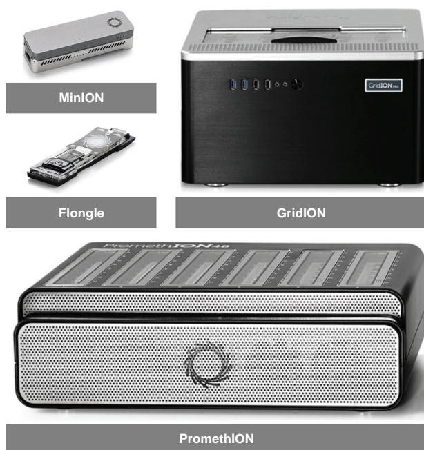
Fig. 2. Oxford Nanopore Long Read Sequencing Platforms. The flagship product, the MinION, is a palm-sized device supporting MinION flow cells containing 4 \times 125 nanopore channels. GridION and PromethION are the higher throughput instruments, supporting 5 and 48 flow cells respectively. The Flongle flow cell contains 126 nanopore channels and is compatible with the MinION and GridION. A flow cell for the PromethION containing 2675 nanopore channels is also commercially available. Instrument pictures from the manufacturer's webpage ( https://nanoporetech.com/ ).
