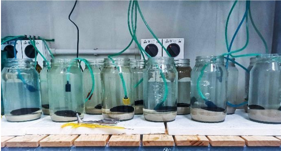
Fig. S1. Laboratory trial set-up for testing thermal tolerance in gravid Echyridella menziesii and E. aucklandica .
