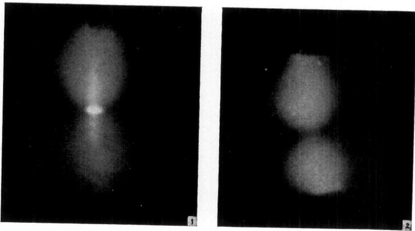
Fig. 1.—Radial contraction of an arc discharge at a low melting point anode.  $\times 15$ .
