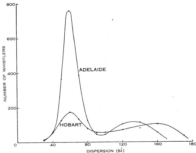
Fig. 1.—Frequency distribution of whistler occurrence versus dispersion for Adelaide and Hobart (1957, 1958) (multichannel analyser data).
