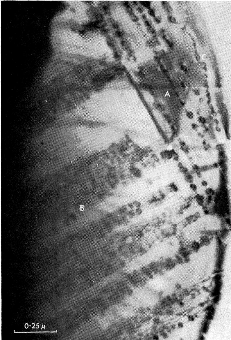
Damage-decorated line defects (A) and plane defects (B) in amethyst. Both types of defect were subsequently identified as Brazil twin boundaries. The irregularly shaped decorated line at C is probably a dislocation.
