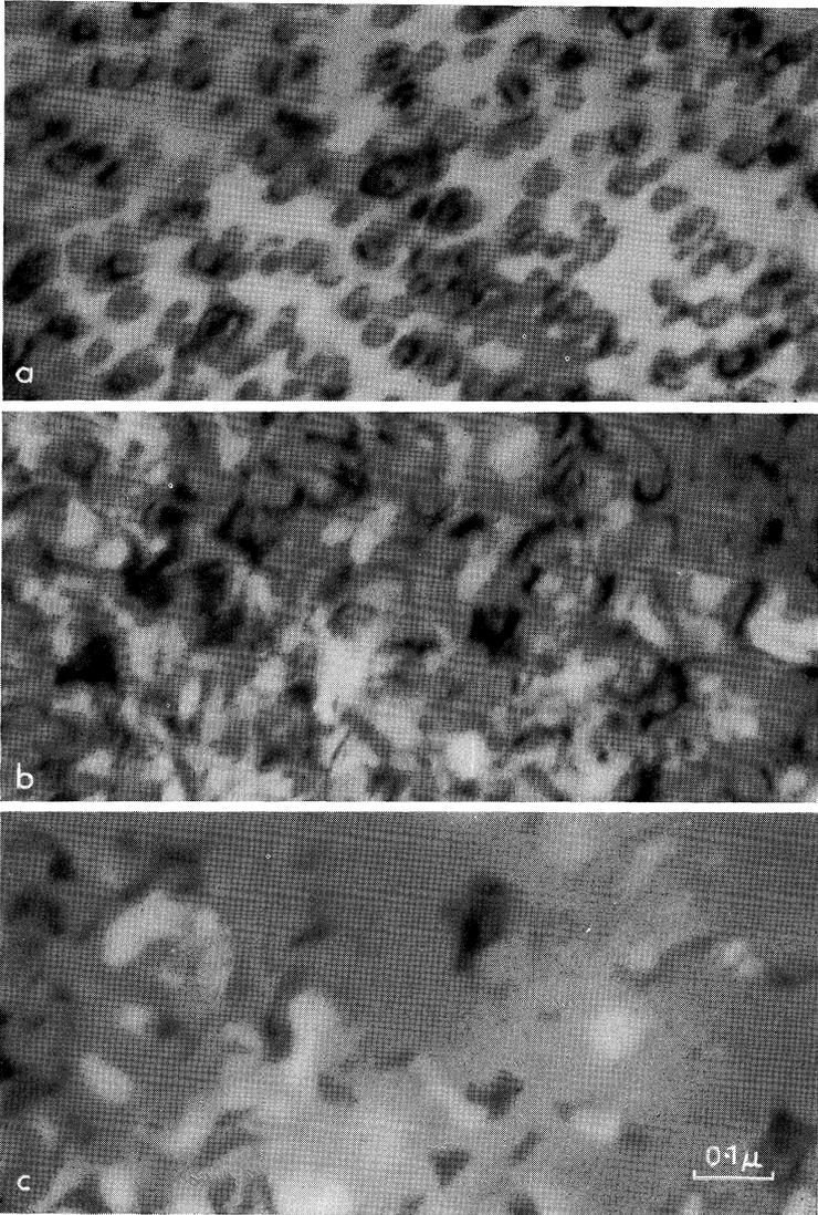
The successive stages of the damage produced in amethyst during observation in the electron microscope. (a) Loops formed after a few minutes; (b) coalescence of the loops; (c) disappearance of diffraction contrast due to transformation to the amorphous state.
